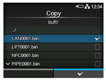
3. After you select the file, press the **\text{\text{Test}}** button to copy the selected file to the USB memory.
