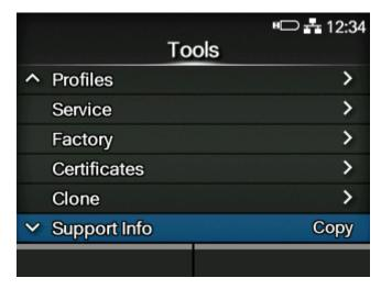
Save various information about the product, such as attached options, serial number, application versions and settings configuration, in a text file (.txt) to the USB memory.
