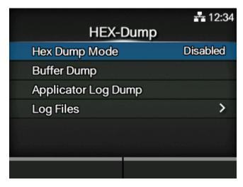
Switches to the HEX Dump Mode, saves the received data and the applicator's log files, and manages the product's log files.
